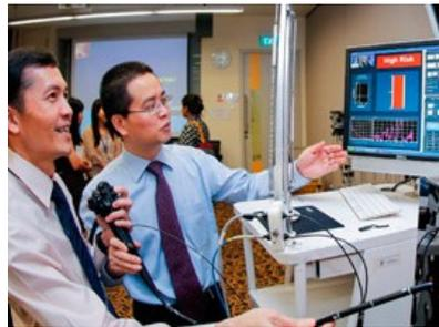
The novel endoscope technology is being marketed as a world first. Instead of taking tissue samples and waiting for lab tests, physicians get an instant diagnosis and make timely medical decisions during routine endoscopic examinations – speeding up the treatment of diseases where early detection and treatment holds the key to long-term survival.
