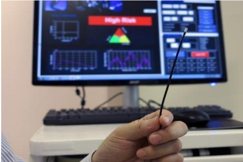
A close-up view of the proprietary confocal fibre-optic probe which enables the collection of biomolecular fingerprint of tissues in less than 1 second.
